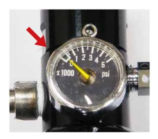
POSSIBLE CAUSE: insufficient air supply ( HPA).
