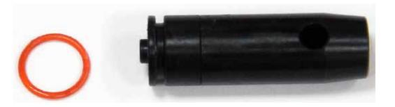
POSSIBLE CAUSE: Striker O-Ring is damaged.
